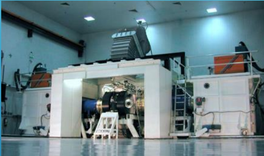
ELECTRA, KrF excimer lézer (NRL) \lambda = 248 \text{ nm} , 300-700 J, 1 Hz-5 Hz rep. rate gáz lézer
